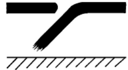
Fig. 14c. Length of seismic zone is the product of rate of underthrusting and time constant for assimilation of slab by upper mantle.
