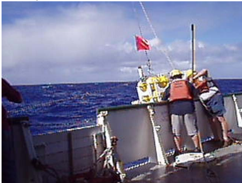
Figure 4. A snapshot during the same recovery as shown in Figure 3. The instrument swayed significantly and just barely missed the hull. One of the tag line holders is a WHOI engineer that came repeatedly to the help of the SIO OBS group who was short in deck experienced personnel.
