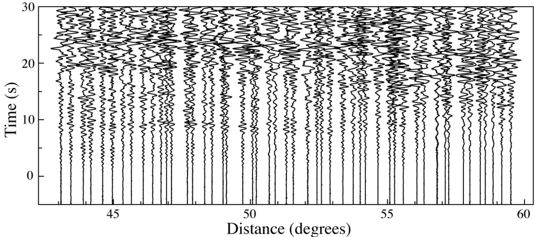
Aligned on theoretical (iasp91) *P*-wave travel times
