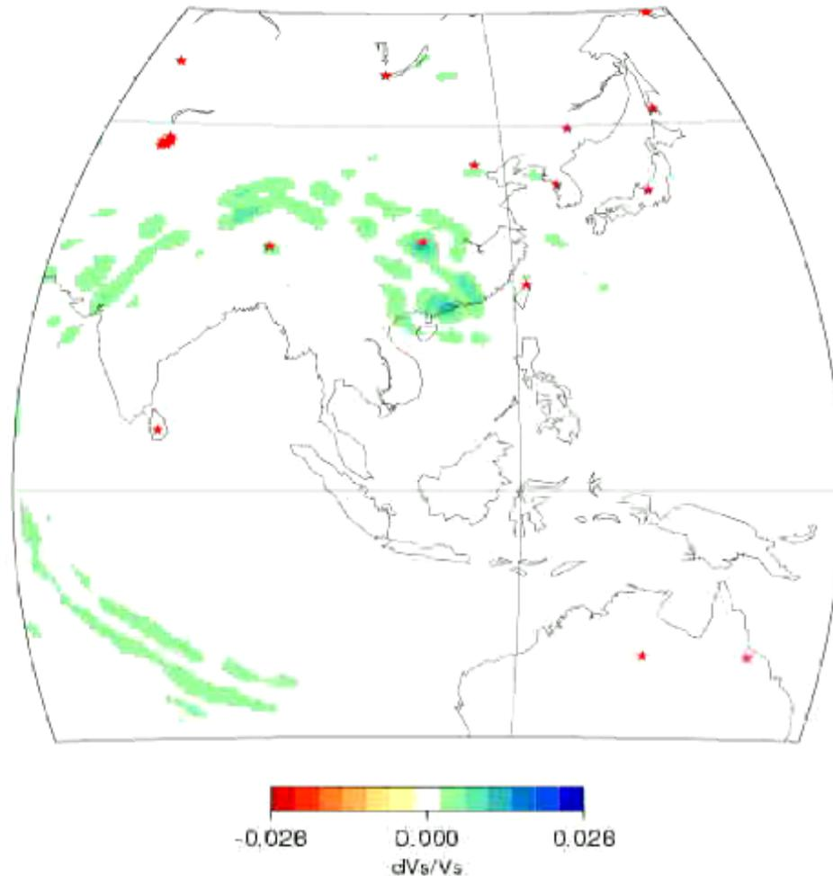
Seismograms from 165 global stations sent back in time using normal mode Green's functions ( $> 150$  s period). Image is mainly of surface waves.
