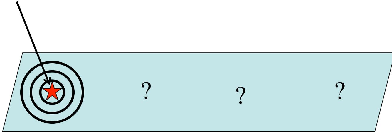
The seismic radiation from the rest of the rupture arrives later in the seismogram.
