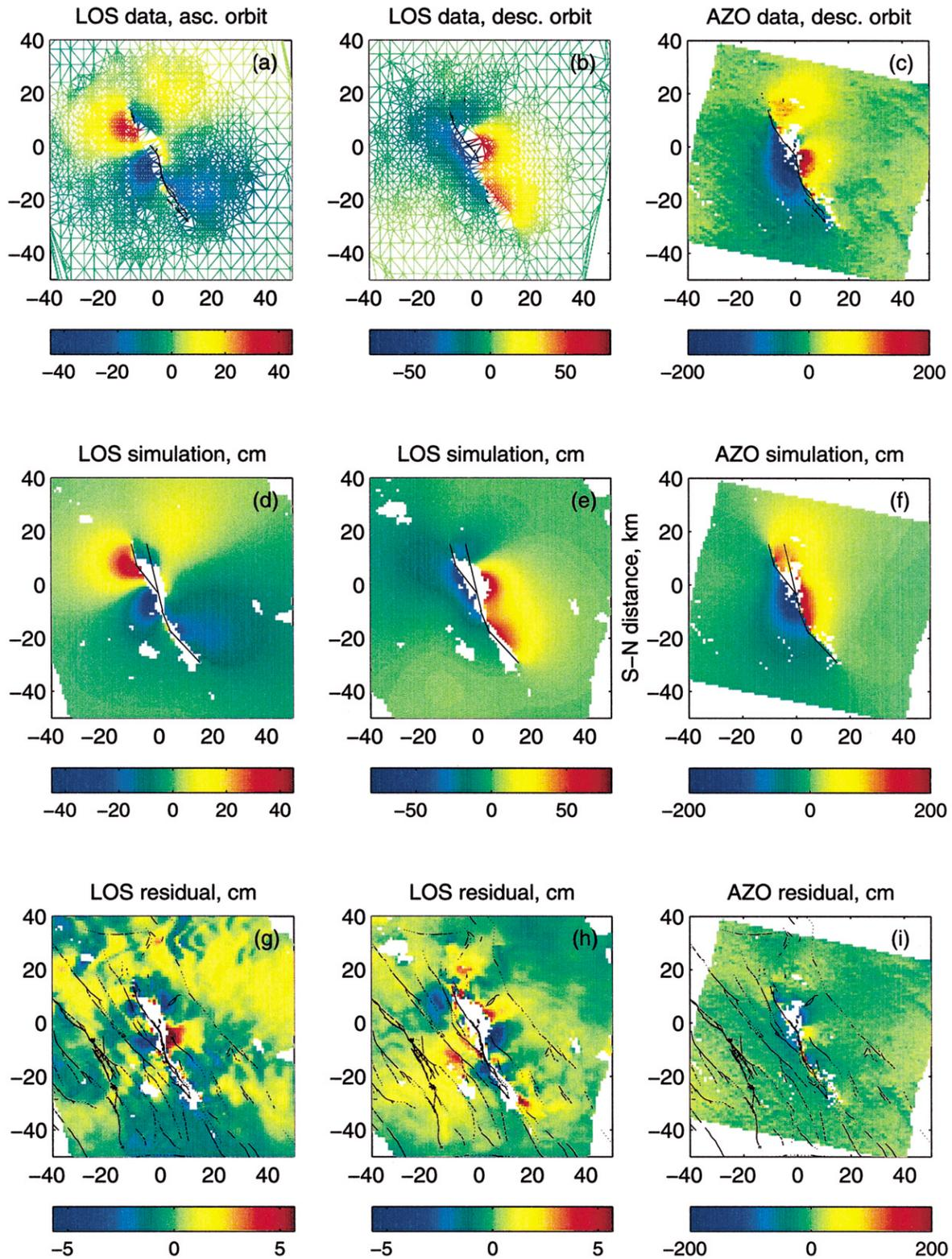
Figure 9. (a) and (b) Subsampled LOS phase data used in the inversion (parts of interferograms beyond the region shown are sampled at a base spacing of  $\sim 10$  km). (c) AZO data. (d)–(f) Best-fitting models. (g)–(i) Residuals after subtracting the models predictions from the data. Note the change in color scale for (g) and (h). In (a)–(i), the origin corresponds to the earthquake epicenter ( $116.27^{\circ}\text{W}$ ,  $34.595^{\circ}\text{N}$ ).
