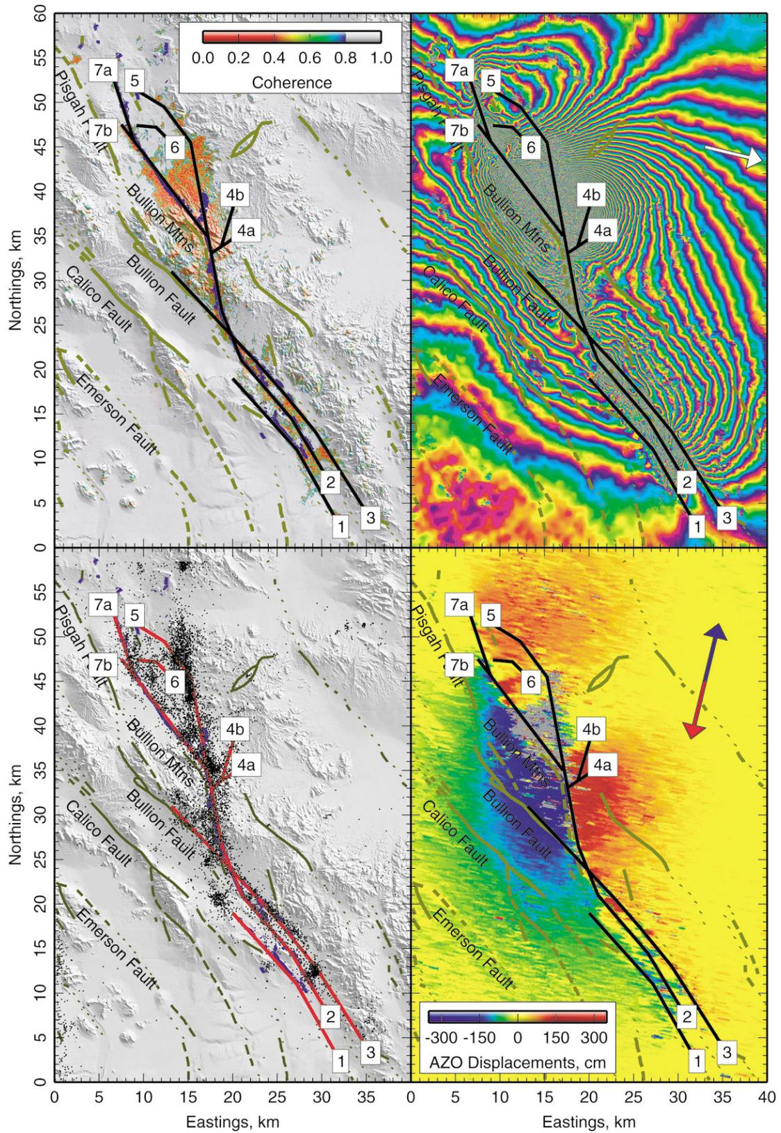
Figure 6. Primary inferred fault segments. Segments are shown with coherence from IPI (top left), the IPI interferogram (top right), relocated seismicity for all of 2000 (Hauksson *et al.*, 2002) (bottom left), and the azimuth offsets from IPI (bottom right).
