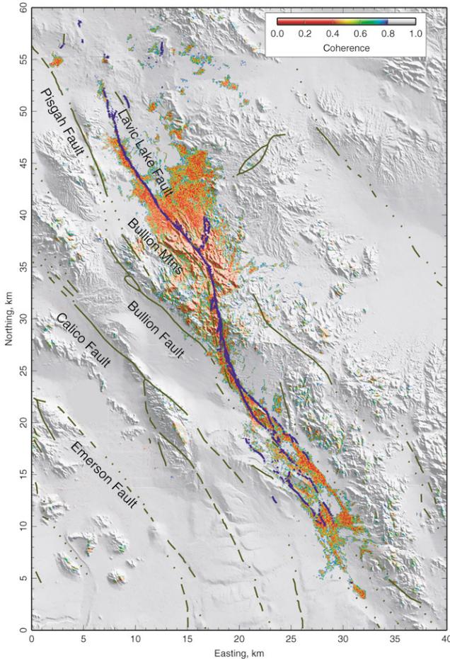
Figure 2. Interferometric coherence,  $C$ , for IP1, with  $C > 0.8$  set to be transparent. Brown lines indicate known faults (Jennings, 1994). Surface rupture as observed in the field is indicated by the blue line (Treiman *et al.*, 2002). UTM zone 11 projection with origin at (116.457W 34.250N).
