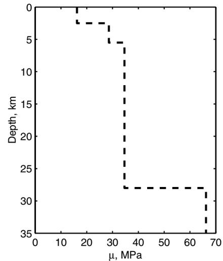
Figure 10. Rigidity structure derived from Jones and Helmberger (1998).
