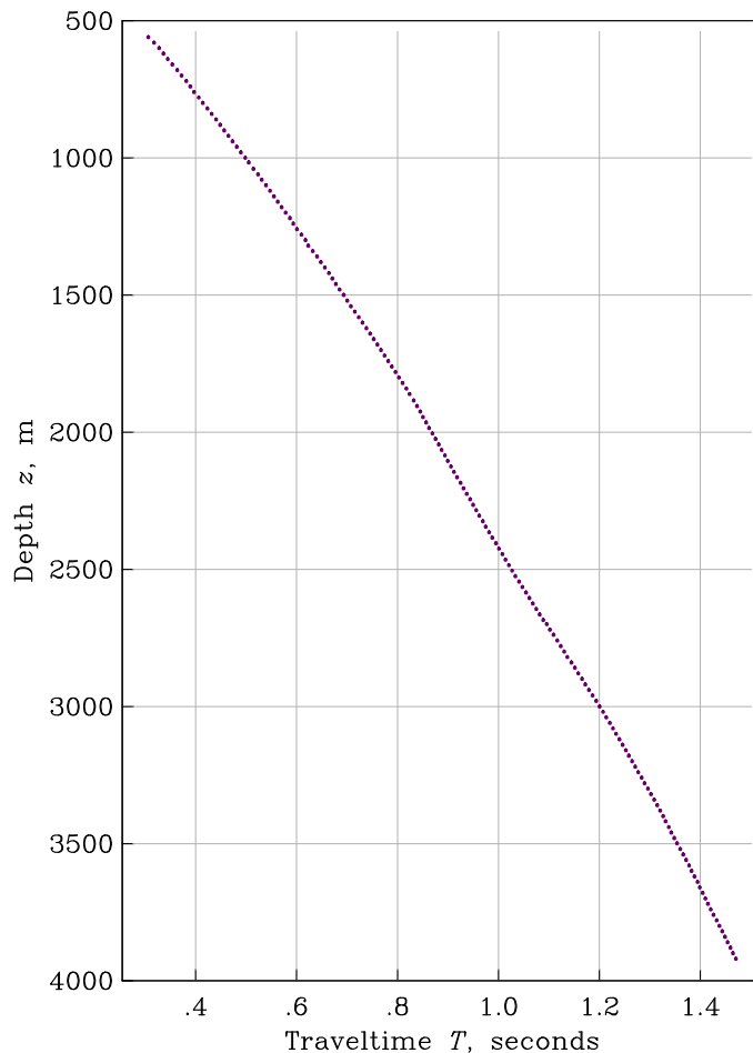
Figure 12.2: Travel-time picks from geophones in a well: the check-shot data.
