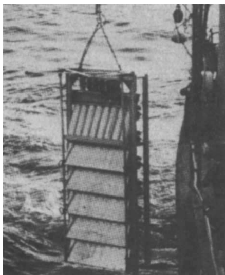
Fig. 2 The explosives platform of the DETES seismology apparatus used by Purdy and co-workers for high-resolution studies of young oceanic crust. (From ref. 1.)
