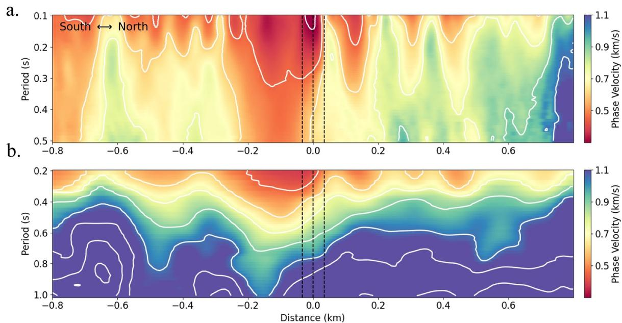
**Figure 2.** Dispersion curves from the active source experiment (a) and ambient noise cross-correlations (b) along the purple segment of the array in Figure 1. Black dotted lines show locations of mapped strands of the Garlock Fault where they cross the velocity profile.
